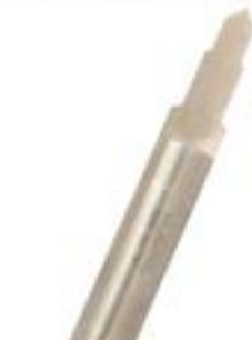
Rod chaged into Multi-step Drill 圓棒改成多段鑽
