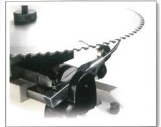
Saw Blade Tip Positioning Device 鋸先端位置決め装置
